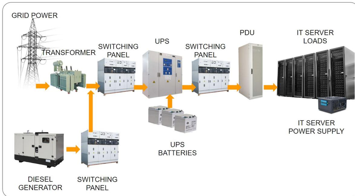
The primary source of power at the data center is typically the local power grid. In case of a grid power interruption (which is not so uncommon in India), a provision of backup power source is mandatory. This is fulfilled through a DG power plant set-up within the data center premises. This also includes on-site storage and handling of fuel (diesel) with underground tanks and network of pipelines connected to the DG room.
