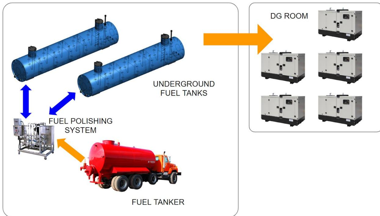
FIGURE 2 : Fuel Management System Layout & Key Components
